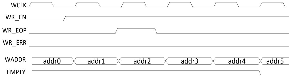
Figure 7-14 Write Timing to Empty FIFO with Rewrite Function
