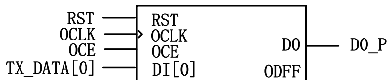
Figure 2-60 ODFF Functional Diagram
