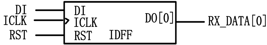
Figure 2-15 IDFF Functional Diagram
