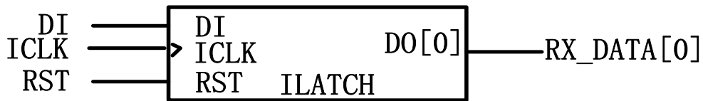
Figure 2-17 ILATCH Functional Diagram
