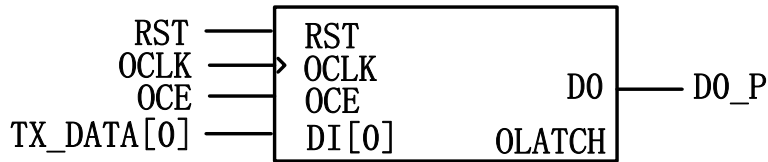
Figure 2-62 OLATCH Functional Diagram
