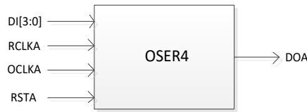
Figure 3-11 OSER4 Functional Diagram
