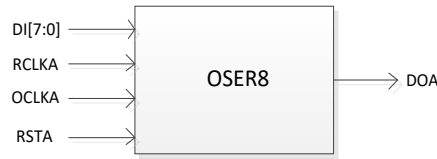
Figure 3-15 OSER8 Functional Block Diagram
